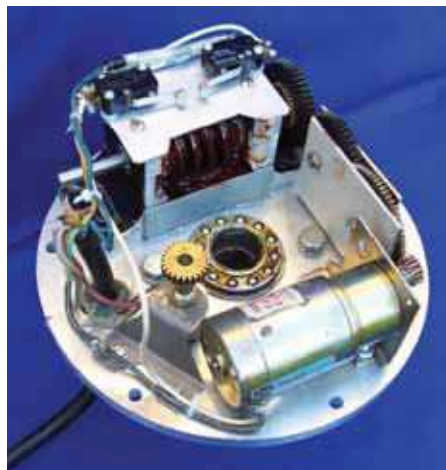
PHOTO 2: The base plate holds the motor, gear train and feedback pot.
