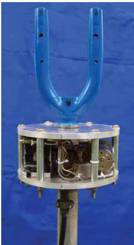
PHOTO 1: General view of the completed rotator, less covers.
